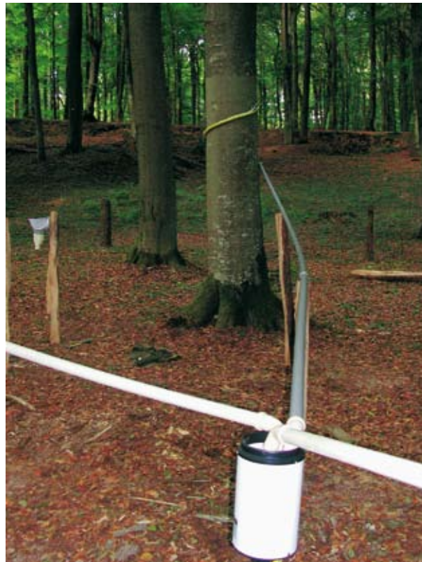
Stemflow and throughfall measurement device in the Huewelerbach experimental plot.
