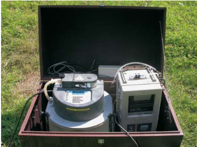
Figure 1: Measurements site at Kaundorf (Raingauge, Flowmeter and Sampler)
