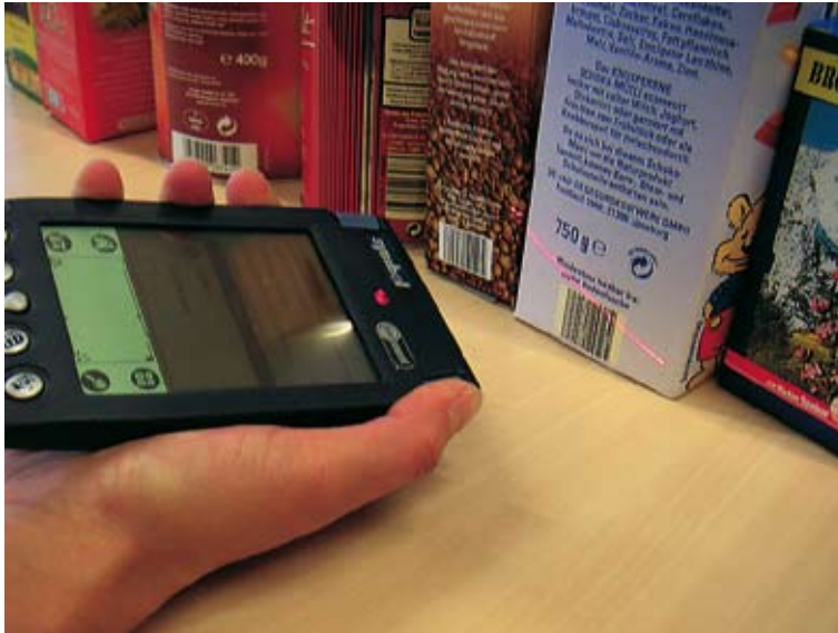
Personal Allergy Assistant (PAA) identifies a food product with its integrated laser barcode scanner
