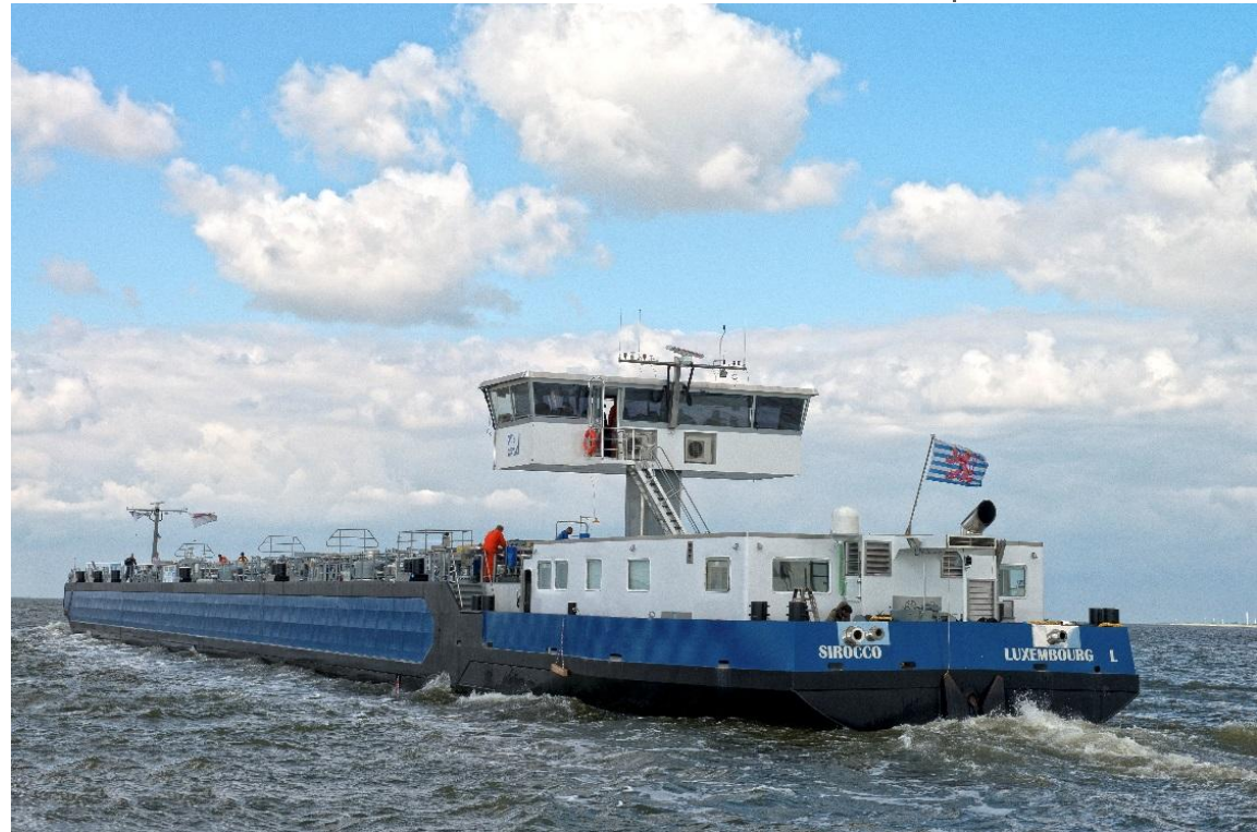
Sirocco, a 110-meter LNG-diesel dual fuel Inland type C tank barge, 1 st dual fuel LNG/DIESEL Tanker, double hull, independent tanks
