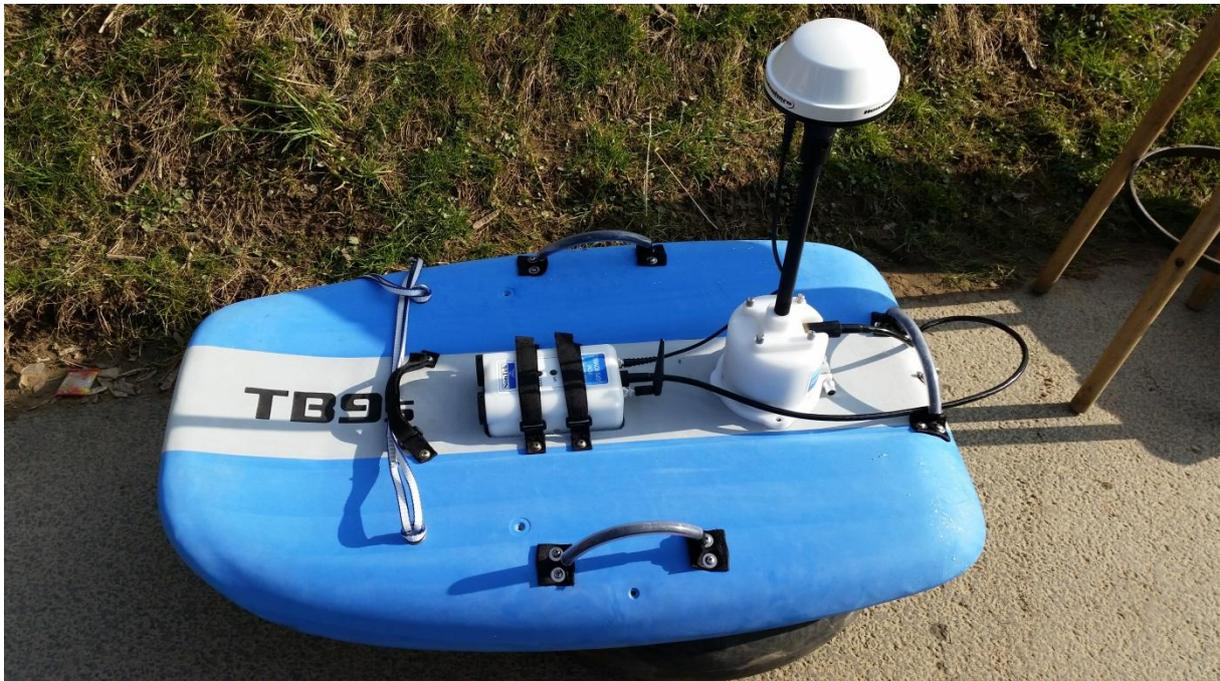
Appareil de jaugeage SONTEK Riversurveyor M9
