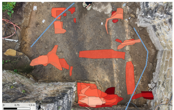
Figure 1: Radar interpretation synthesis of wall features and possible pipes across all investigated depths, combined with an orthophoto of Planum 1 at the artillery tower in the outer bailey of Beaufort Castle. The darker colour shades indicate higher depths compared to the brighter ones.
